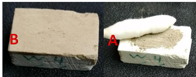
Figure No. (5) shows the result of using the lipase enzyme loaded on the pure Faker polymer and nano-silica in cleaning the surfaces of the limestone wall inscriptions of the second sample, where (A) shows the dirt and (B) the result of cleaning.
