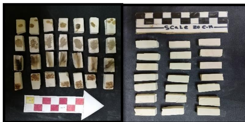
Figure No. (2) shows the preparation of limestone inscription samples for experimental study
