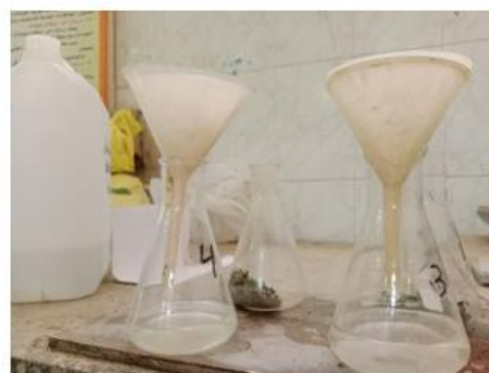
FIG 6. The filtration process for the concrete solution
