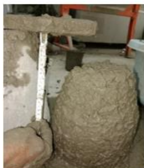
FIG 2. Slump Test Measurement
