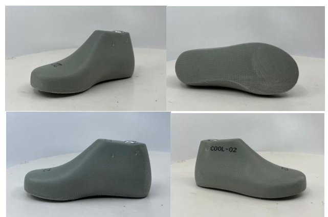
Figure 9. Developed mold for ages 2-5
