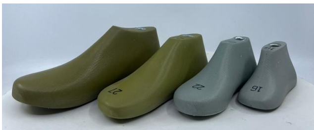
Figure 3. Size-based molds design
