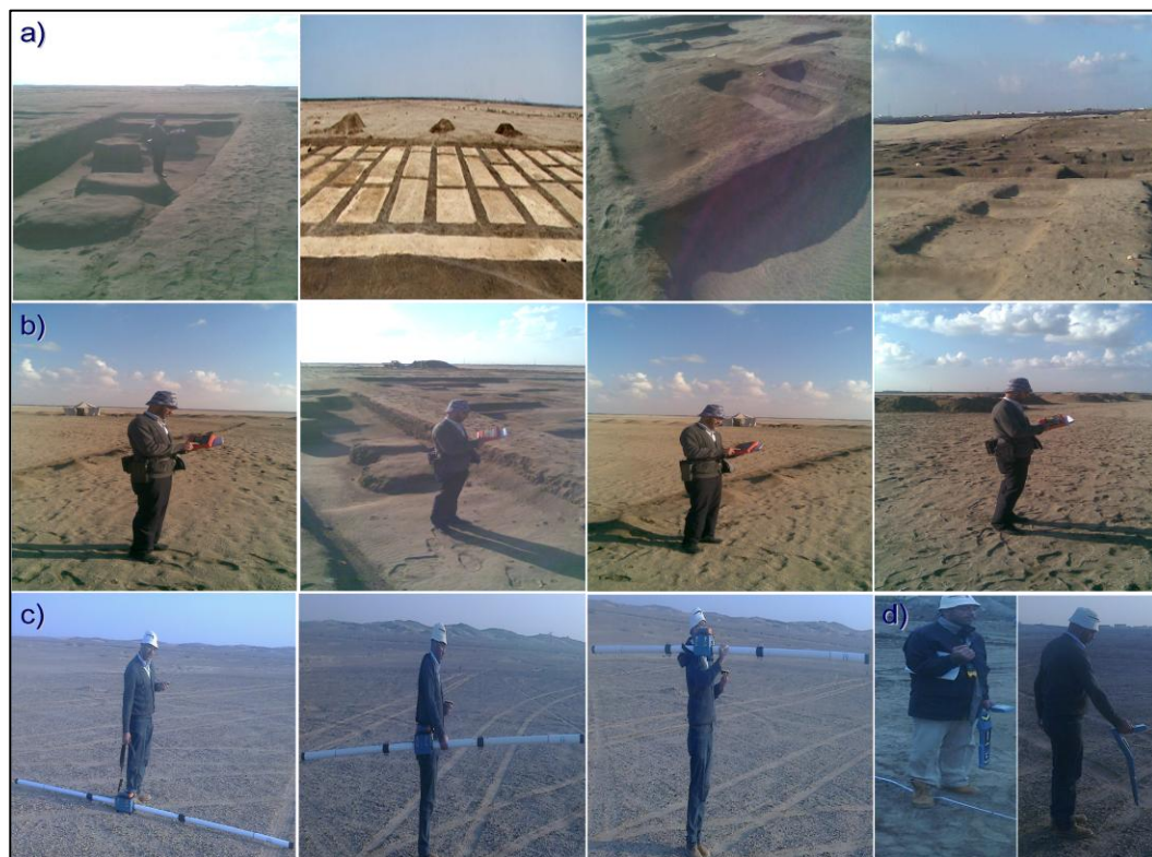
Fig. 2: Field photographs showing a) the excavation countryside at 'Tell Hebua' archaeological site and b) the measuring systems Geonics 'EM-31-MK2', c) ABEM 'WADI™ VLF-EM' and d) RadioDetection 'RD-8000'.
