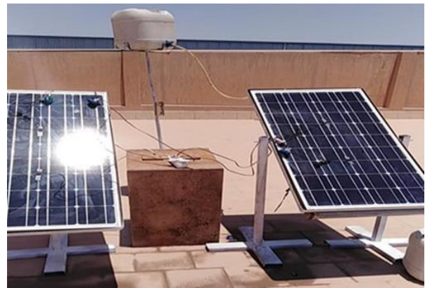
Figure 2: Face of two PV panels with 30° angle of inclination with horizontal, one with cooling system and the other without cooling system.
