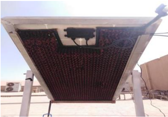
Figure 4: Close back to PV panel with Cooling Pad.
