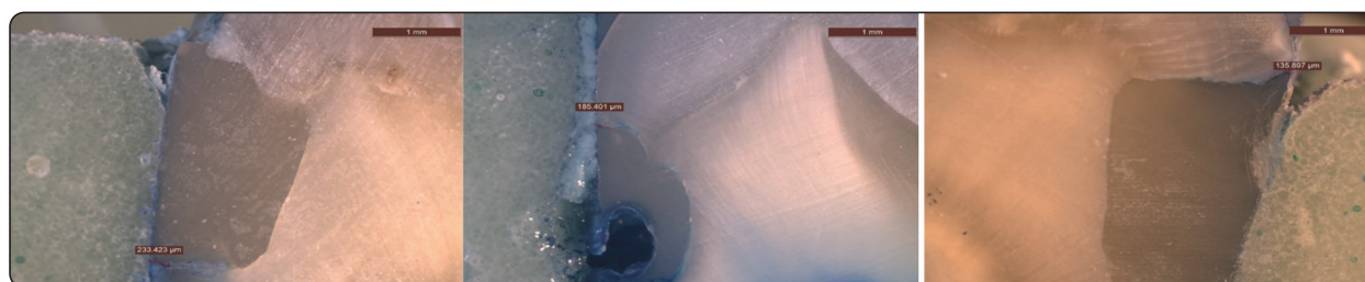
Fig. (5) Stereomicroscope image of G-aenial Universal injectable composite showing depth of Methylene Blue dye penetration in class V cavities at tooth restoration interface using image analysis software.
