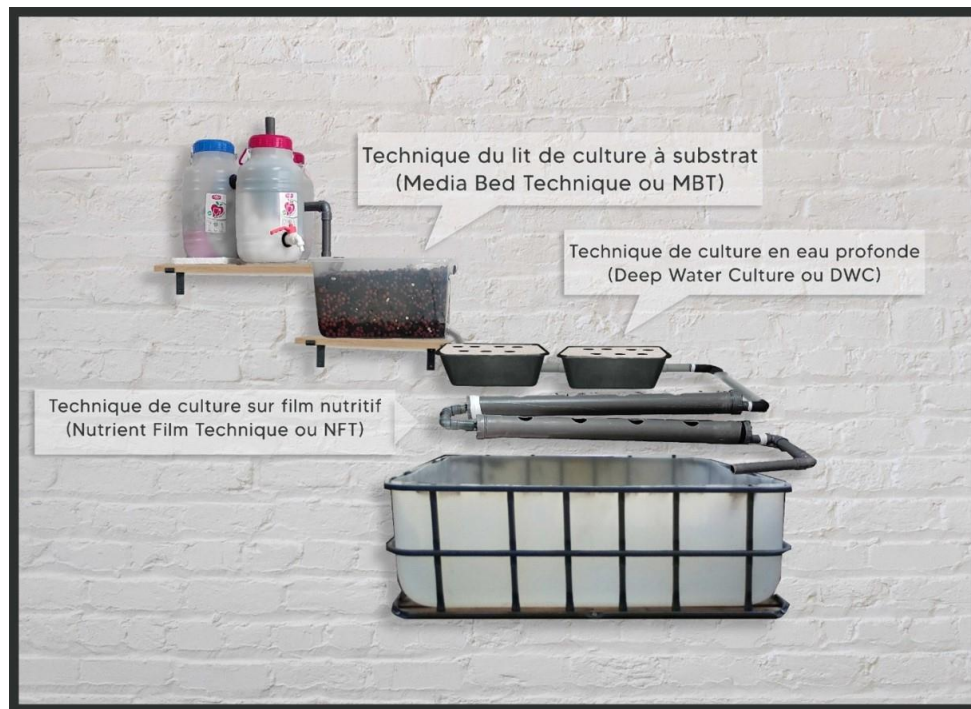
Fig. 1. Sketch of aquaponic system used in experiment
