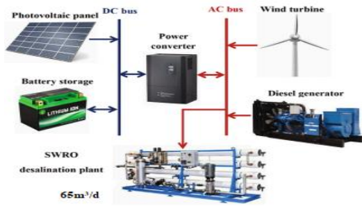
Figure 1: proposed RO unit hybrid energy system
