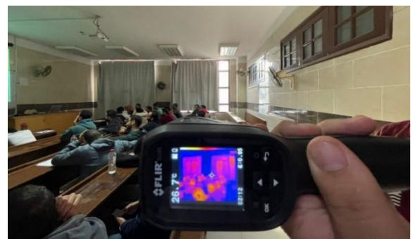
Figure 2: Dual perspective of the lecture room and thermal camera capturing the temperature distribution inside the lecture room.
