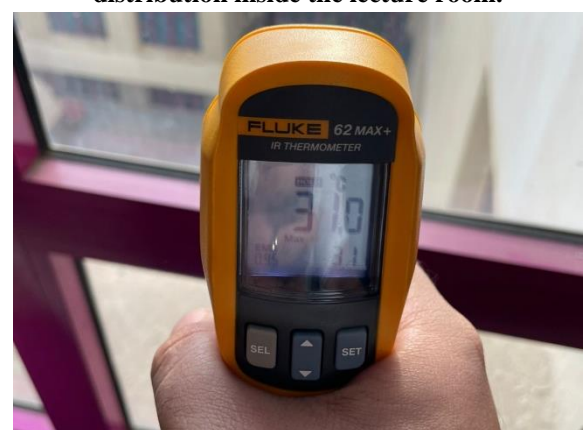
Figure 3: Measuring lecture large windows temperature during winter season using IR thermometer
