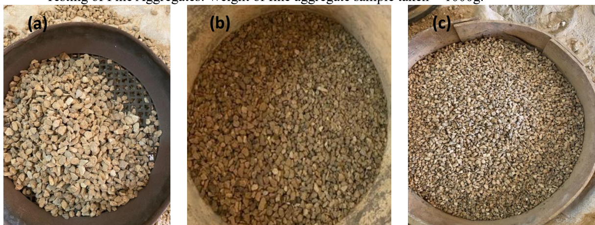
Fig. 2. Illustrates three different aggregate gradations : (a)N.M.S 10 mm, (b)N.M.S 15 mm, and (c)N.M.S 20 mm.
