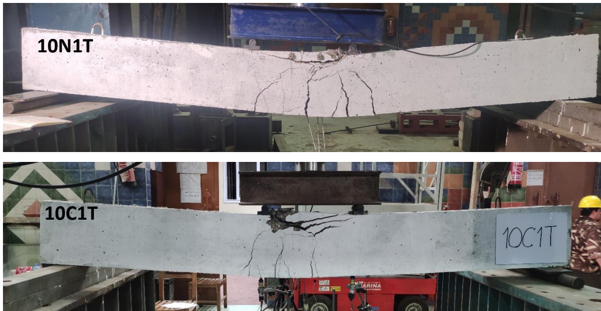
Figure. No. 6: Cracks of Specimens 10N1T and 10C1T at Failure
