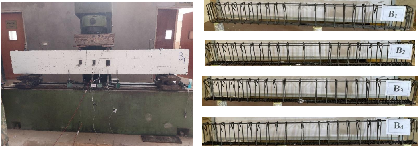
Fig. 3. Experimental test setup and steel arrangement of beams B1, B2, B3, and B4.
