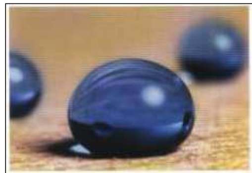
Fig.2. Wood Can be given an. extremely water-repellent self-cleaning surface.
