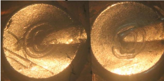
Figure 2: .22" test fired cartridge (Lt) and exhibit (Rt)
