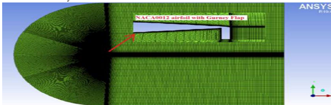
Fig3: Computational domain of NACA0012 Airfoil with GF.
