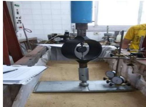
Fig 2. Loading System installation
