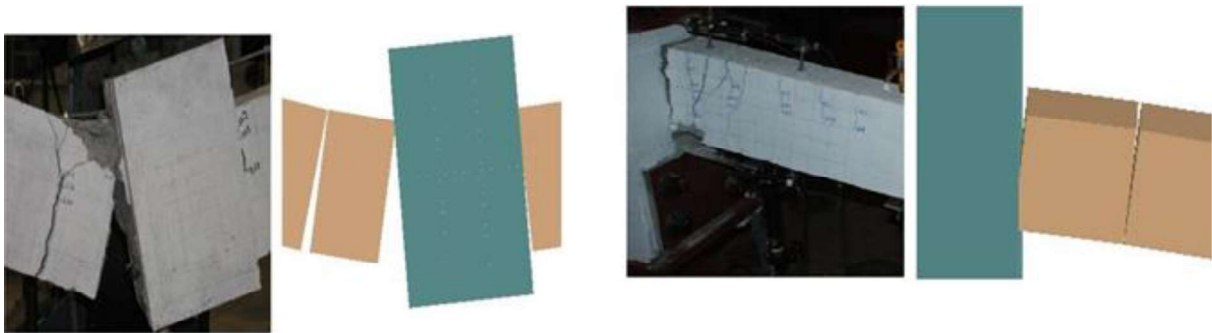
Fig 11: Observed and Predicted Crack patterns for Specimens S1
