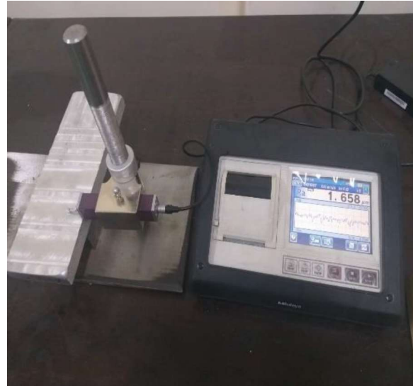
Figure.2 SJ-310 SurfTest tester
