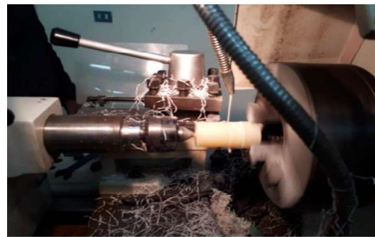
Fig 3. The machining of epoxy/TiN nanocomposite specimens during turning.
