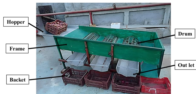
Fig. (1): A Photo of the manufactured grading machine.
