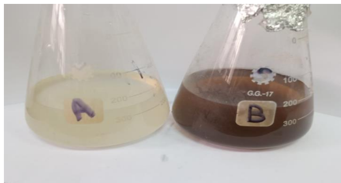
Fig. 2. Biosynthesis of AgNPs by Trichoderma harzianum A: Aqueous fungal extract. B: AgNO 3 solution with aqueous fungal extract after incubation
