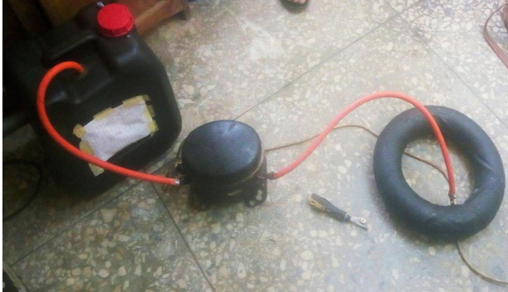
Fig. (2): Set up of the fittings of the laboratory scale digester with compressor.
