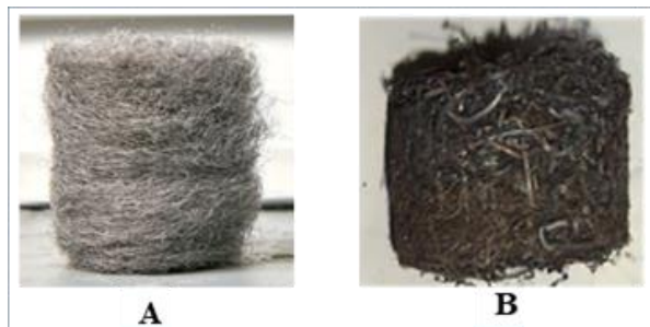
Figure3. Photos of steel wool, (A): Before absorbing H 2 S, (B): After absorbing H 2 S.
