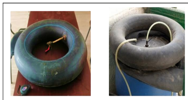
Figure 1. Raw Biogas collection by tyre tube
