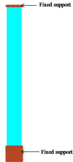
Fig. 7: Fixed Supports Condition of Column [7].
