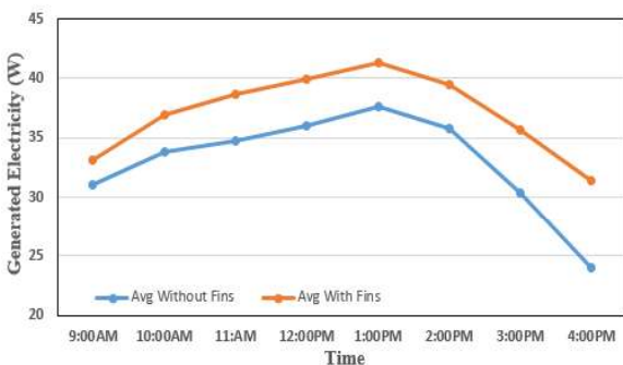
Fig 4: Average Generated Electricity for PV with and without fins systems during the daytime in August 2018.
