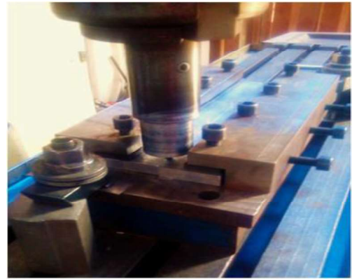
Fig. 1 Friction stir welding process.
