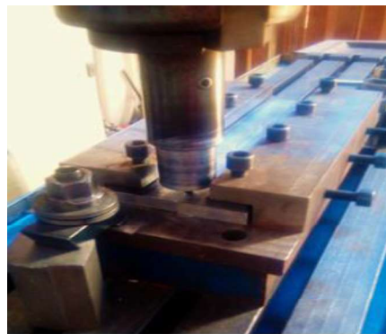
Fig. 1 Friction stir welding process
