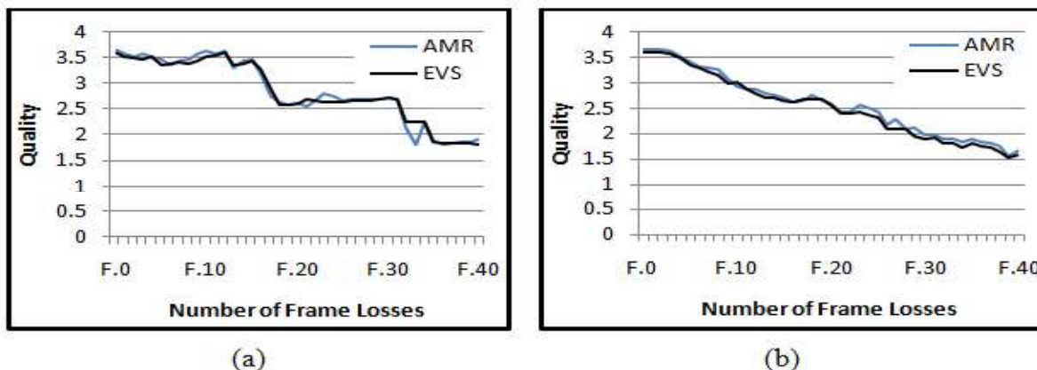
Fig 8: Average Quality of EVS and AMR codec, in case (a) Continuous and (b) Discontinuous Frame Loss for an Arabic Male.
