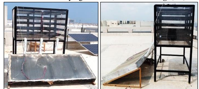
Fig.(2.3): Solar collector and drying chamber.
