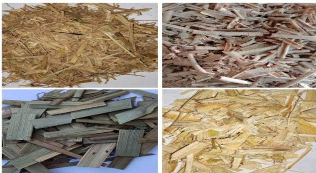
Figure .1. Raw materials rice straw, sugar cane waste, date palm waste and sawdust.
