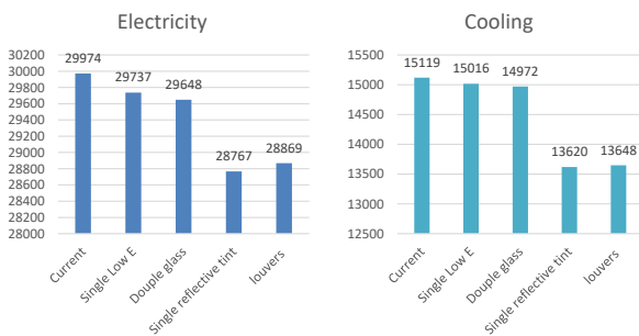
Fig.15: Simulation results of heat gain, energy consumption, and annual cooling loads for the proposed glass alternatives Source: Author
