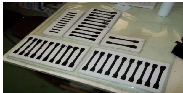
Fig. 6 the specimens in the silicon rubber molds.
