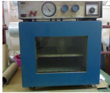
Fig. 4 Oven and vacuum chamber.
