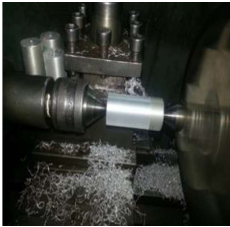
Fig 2. The turning process carried out on Al-Si/MWCNTs nanocomposites.
