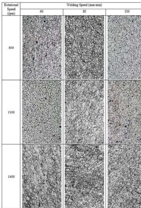
Fig (6). Microstructure at the center of DRZ for AA6061-O samples FS welded using different tool rotational and welding speeds ( \times 100 ).
