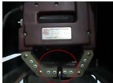
Fig (1) : The electromagnetic yoke coil placed around the candle flame.
