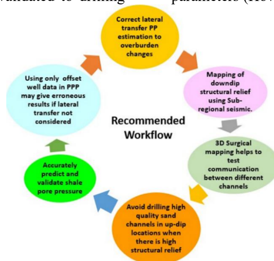
Fig. 4. Recommended workflow to avoid missing the potential for lateral transfer (centroid) of overpressure.
