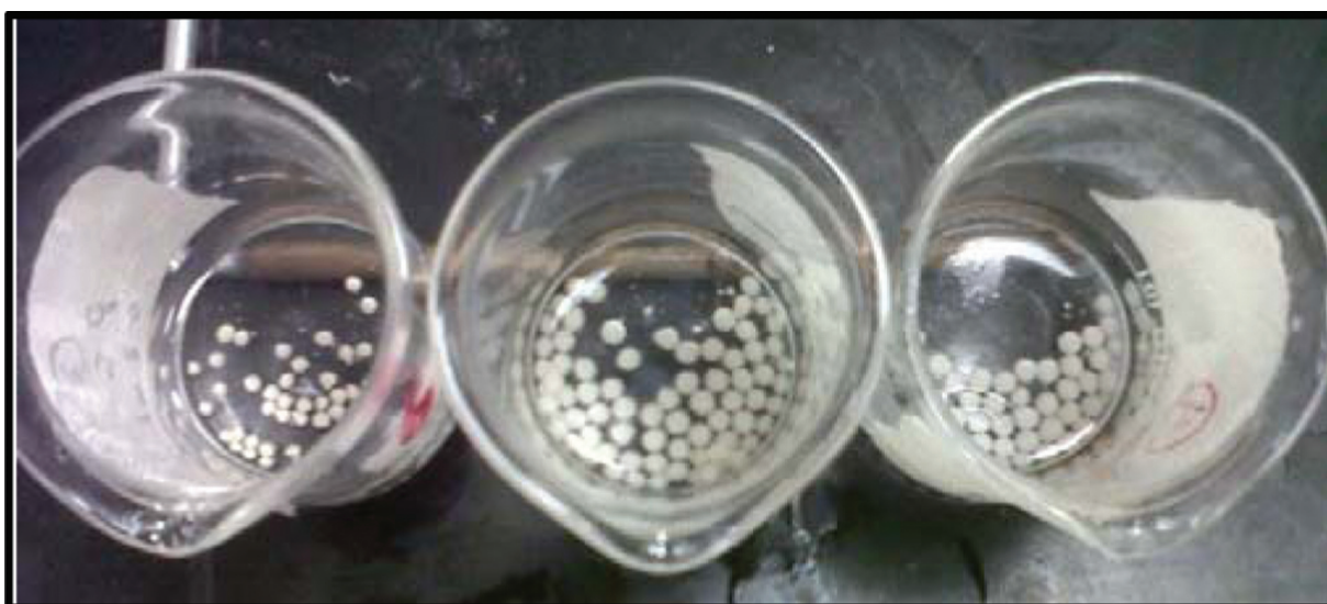
Alkaline protease production of free and immobilized (in alginate beads) cells of Bacillus sp. strain NPST-AK15 in repeated batch bioprocess.
