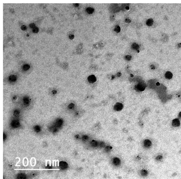
Transmission electron microscopy image of alginate-loaded peppermint nanoformulation.
