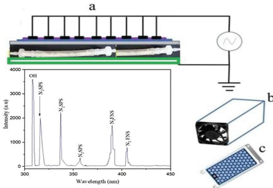
SDBD (a) electric circuit, (b) Teflon box, (c) honeycomb configuration [22]. SDBD, surface dielectric barrier discharge.
