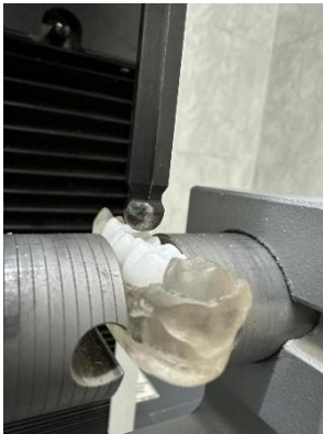
Figure 2. Fracture resistance testing
