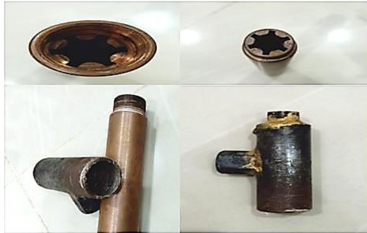
Figure 3: The internal fins and the cap with two opening at the condenser section.
