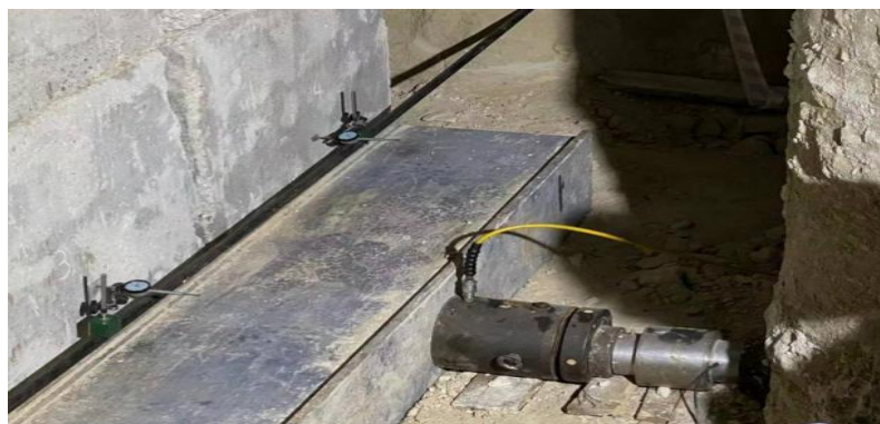
Figure 7: Field photograph of horizontal load testing equipment for the test piles
