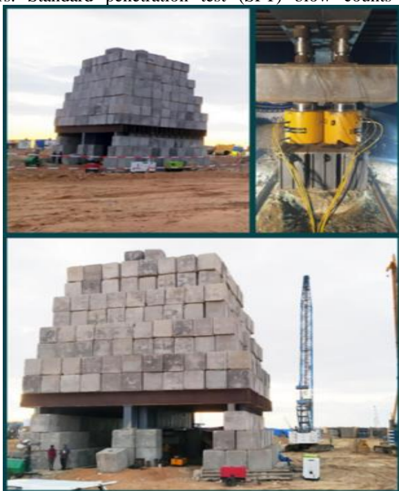
Figure 4: Field photograph of the test pile setup for 1700-ton capacity piles (left) and load test data (right)
