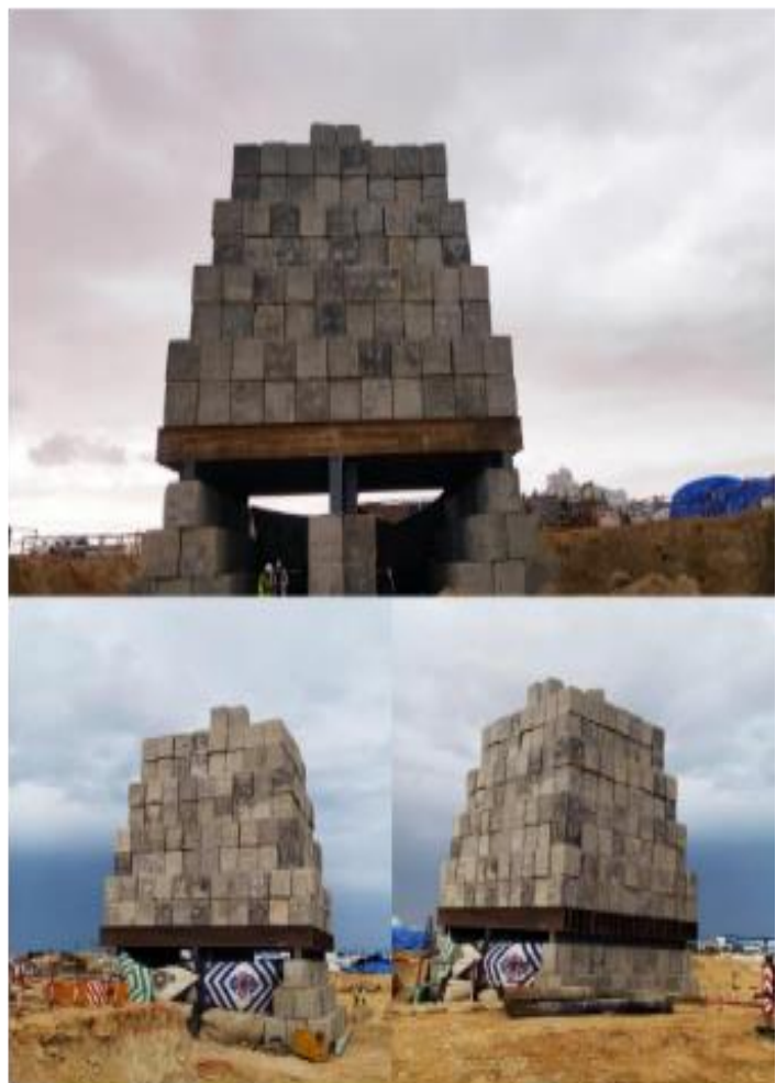
Figure 11: Single pile reinforcement and friction-end bearing resistance test results
