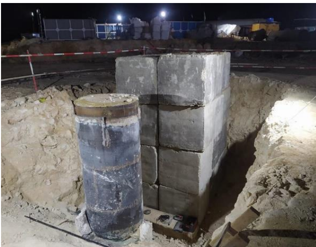
Figure 12: Single pile end-bearing resistance test results
