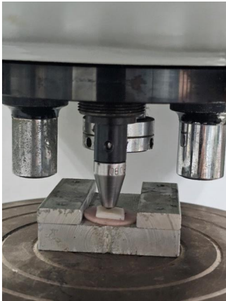
Figure 4: Vickers micro-hardness tester with diamond indenter
