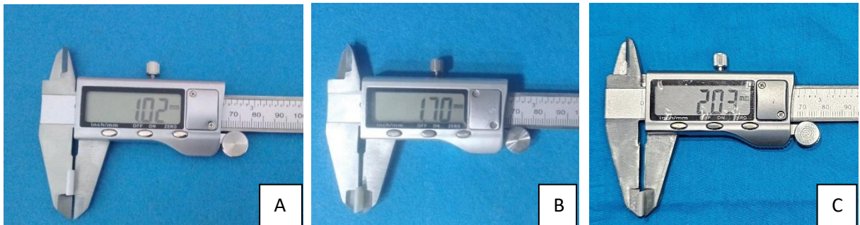
Figure 2: The dimensions of each specimen were verified using a digital caliper, A. After zirconia sintering; B. After dentin firing; C. After enamel firing.
