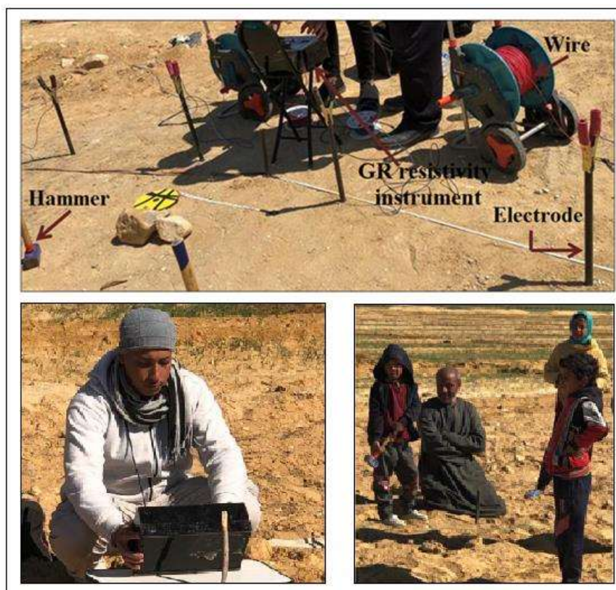
Figure 5: Field photo and resistivity field instruments.
