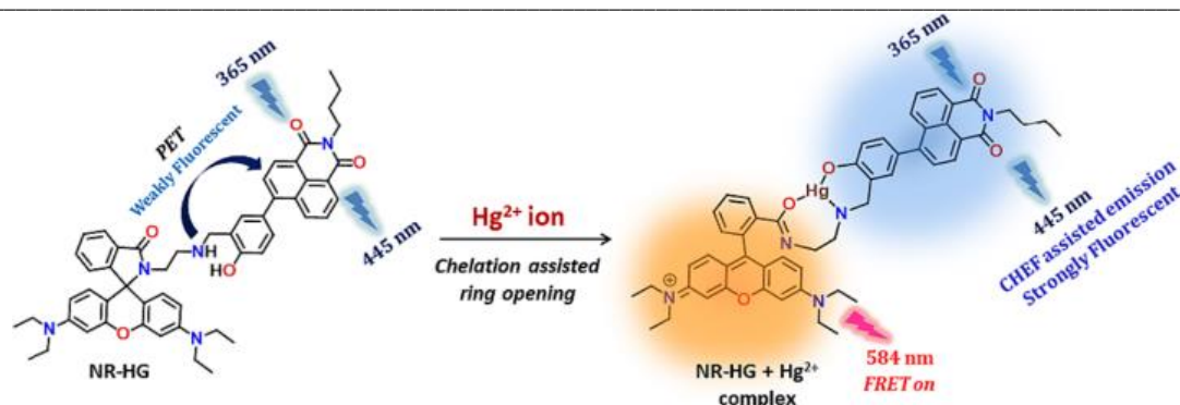
Scheme 15: Sensing mechanism by FRET for NR-HG sensor [92].
