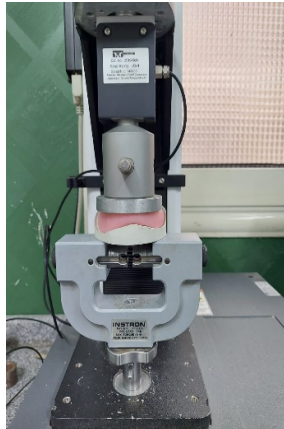
Fig. 2 The whole model tested by the universal testing machine.
