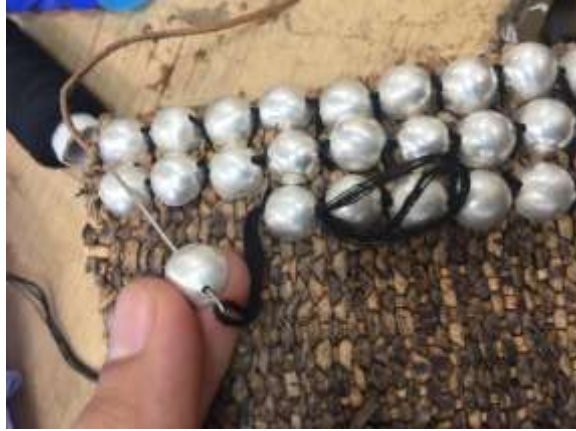
Figure 3-5 Stitching the silver domes above the leather weaving (Photographed by Amal Al-Ismaili, Metal workshop, Sheffield Hallam University, UK, 2017)
