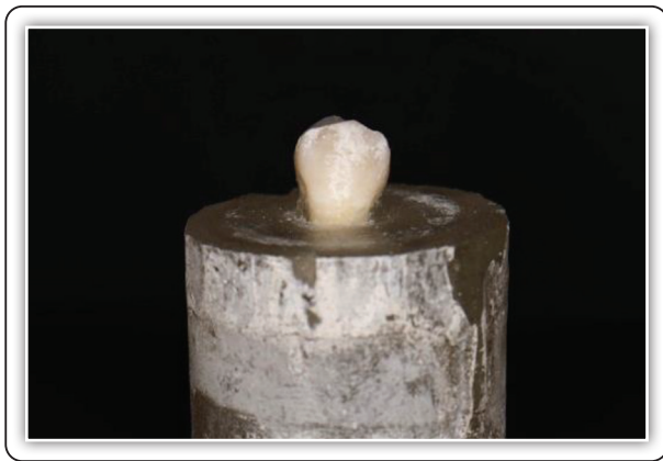
FIG (1) Tooth embedded in self-cured acrylic resin. Uncovered buccal surfaces above the CEJ.
