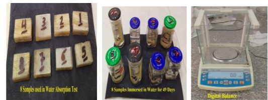
Figure (9) Measuring the mass of the laminated composite specimens using digital balance
