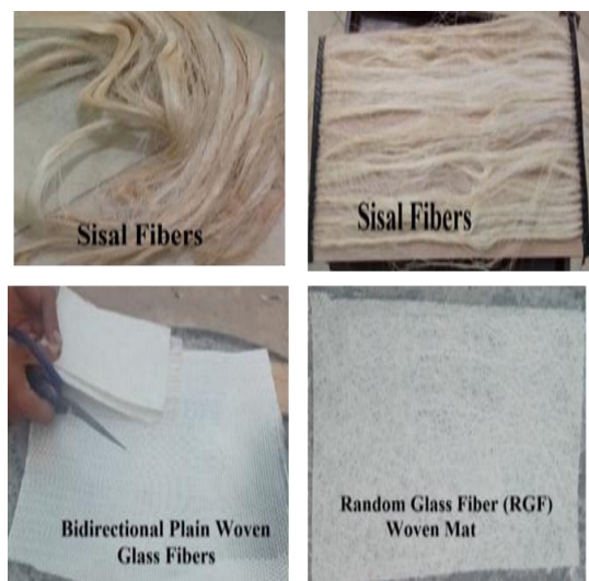
Figure (1): Natural fibers (Sisal Fibers) and Synthetic fibers used in fabrication laminated composite materials
