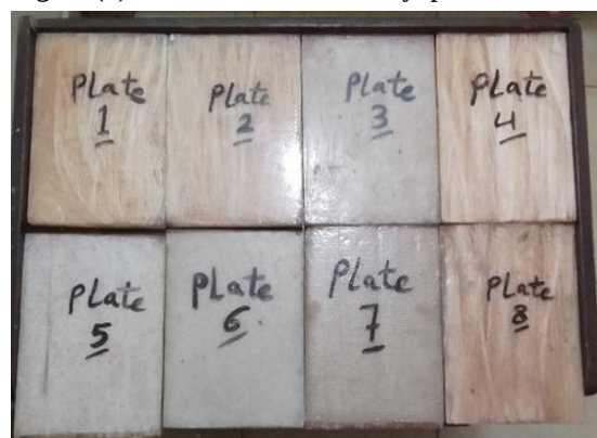
Figure (3) Eight Laminated composite plates Manufactured by hand layup methodology
