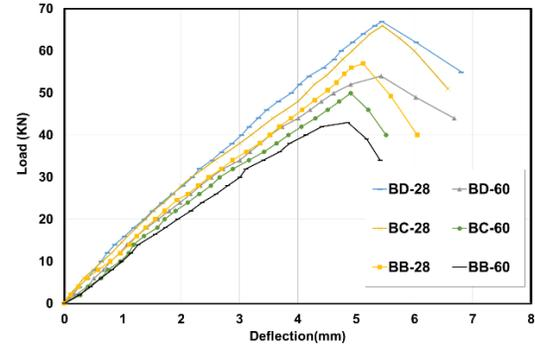
Figure 7- Load versus midspan deflection for test beams
