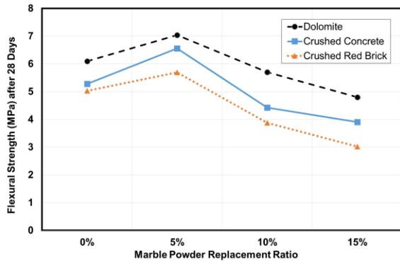
Figure 6- The effect of MP replacement on flexure strength
