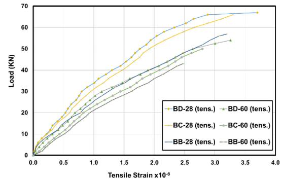
Figure 8- Load versus bottom tensile strain for test beams
