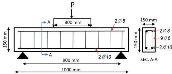
Figure 1- Dimensions and load configuration of test beams
