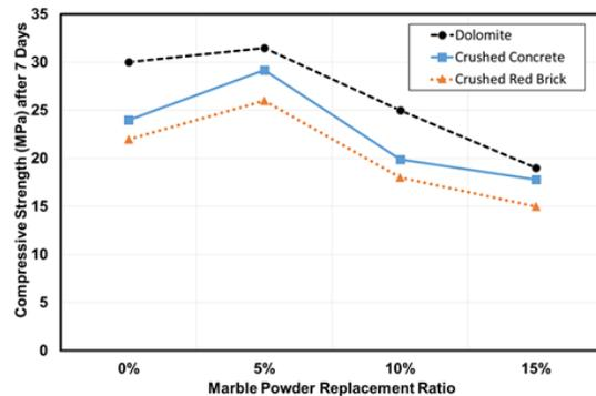
Figure 4- The effect of MP replacement on 7 -day compressive strength
