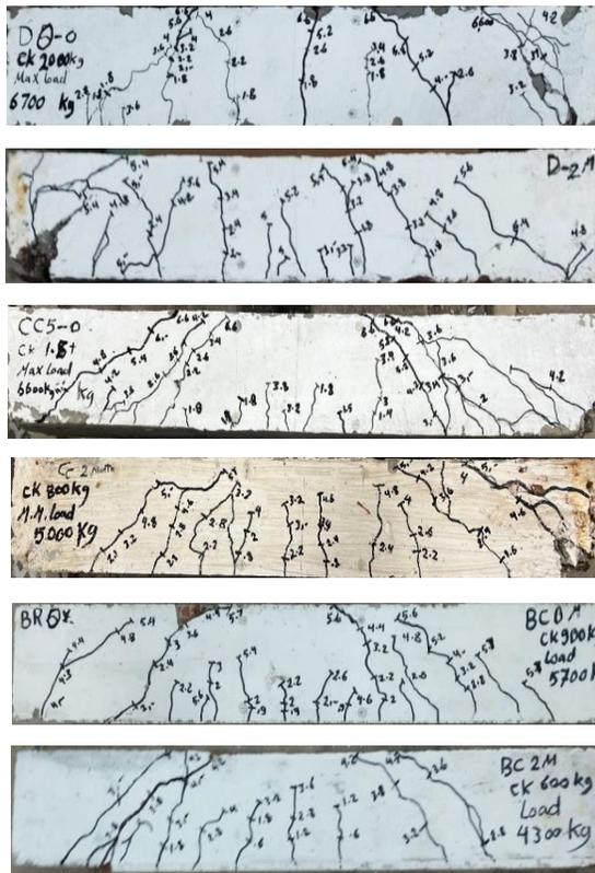
Figure 11- Failure modes and cracking patterns at failure
