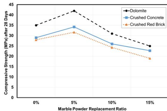
Figure 5- The effect of MP replacement on 28 -day compressive strength
