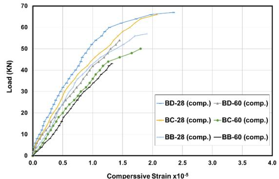
Figure 9- Load versus top compression strain for test beams
