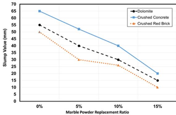
Figure 3- The Relation between slump and marble powder ratio
